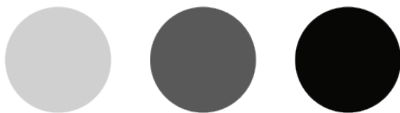
Figure 15.1. Luminous emittance (amount of light emitted by a surface) evokes the sensory modality of brightness. The disks have different emittances and are perceived as having different brightness.
