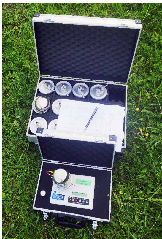
Fig. 15. Radon Monitor-2 (RM-2)
