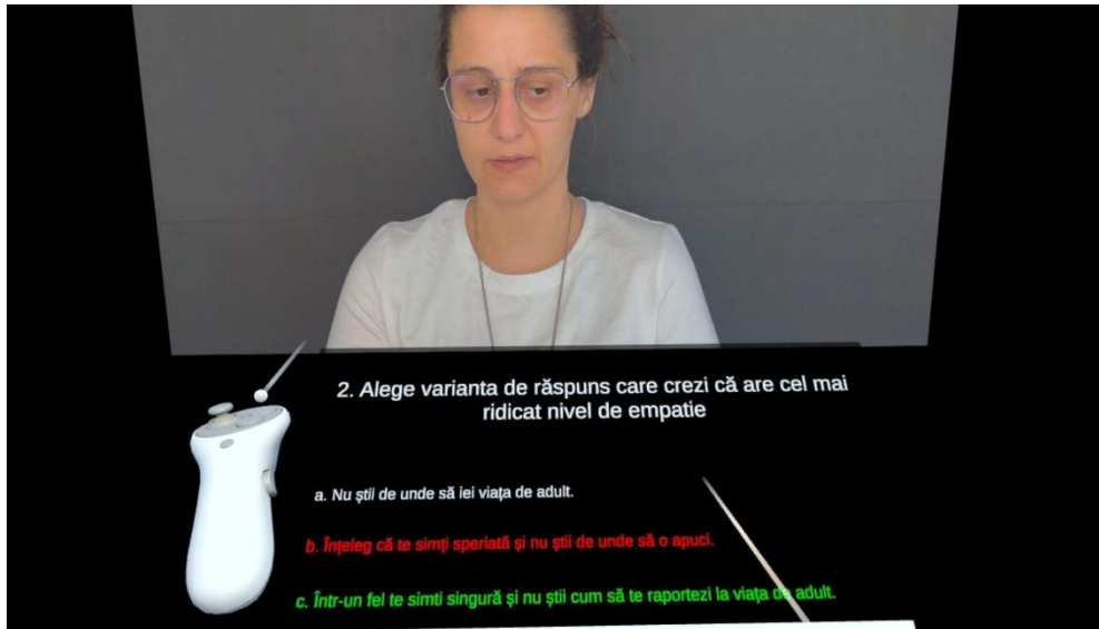
Figure 3. Formative component feedback screen allowing users to review video segments in which incorrect responses were selected, along with the correct choices. The interface is in Romanian.
